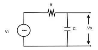
(d) Determine the phase angle  $\varphi(\omega)$  of the output voltage, relative to the input voltage, as a function of frequency (in terms of  $\omega$ , R, and C).
